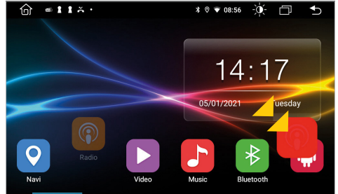
To be able to place a new basic app, you must first create space for it. For example, pull the radio app to the bottom right.
