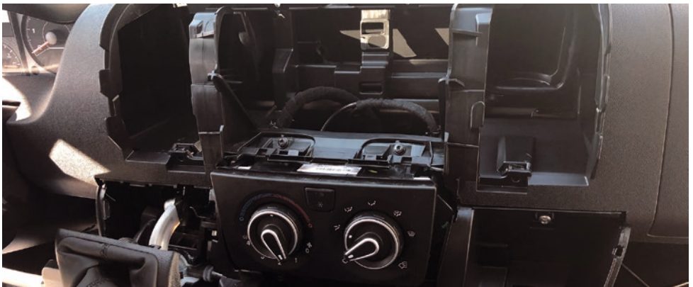
Remove the original panel by lifting it and pulling it forward.
