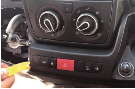
Remove the original panel.
