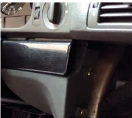
Remove the panels next to the steering wheel and on the passenger side. Now unscrew the screws underneath.
