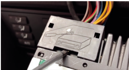
Use the flat-head screwdriver to pry off the radio adapter.
