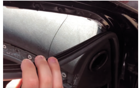
Pull the door seal of the A-pillar to the lower last screw.
