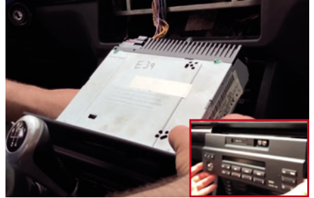
Pull out the original radio.
