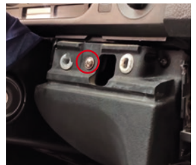
Remove the panels next to the steering wheel and on the passenger side. Now unscrew the screws underneath.
