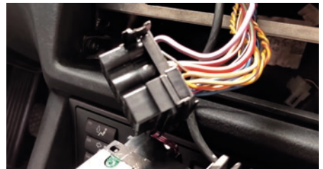
Remove all remaining cable connections on the radio.
