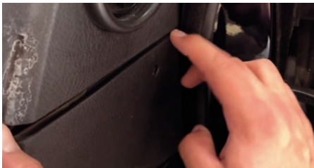
Use the dashboard panels to route the cable in the direction of the center console.
