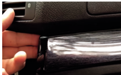
Remove the panels next to the steering wheel and on the passenger side. Now unscrew the screws underneath.
