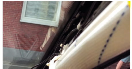
Route the cable of the GPS antenna along the A-pillar.
