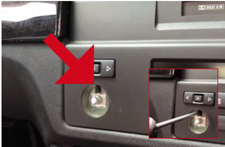
Inside the button is a small screw at the top, which has to be loosened.
