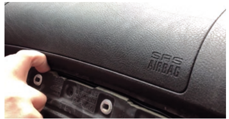
Use the dashboard panels to route the cable in the direction of the center console.
